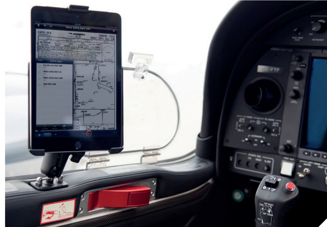
Built-in tablet mount provisions for pilot & co-pilot armrests (tablet and cradle for visual purposes only)
